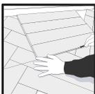
Join together four planks, and using this as a guide scribe mark this into the wall along the whole length with a pencil, as shown below.
