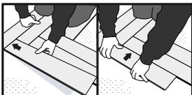
Or by hooking the end under and pulling in the long length. Tapping as necessary to ensure a good connection.
